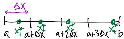
$$\text{Area of rectangles} = (\Delta x) f(x_1^*) + (\Delta x) f(x_2^*) + \dots + (\Delta x) f(x_n^*)$$
